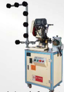
全自动金属上止机(铝丝) Full automatic metal upper stop machine (aluminum wire)
